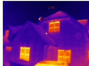
Examples of a thermal imaging photographs with different aged buildings and types of construction, that illustrate the changing standards required by the Building Regulations. Left a building from the 1990s, Below right - our house built in 2003.
